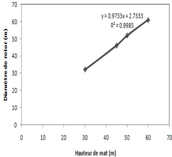
Figure-5: Effect of mast height to the diameter on the rotor [1]
