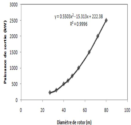
Figure-6: Effect of rotor diameter on the output power [1]
