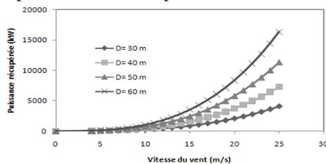
Figure-8: Effect of wind speed and rotor diameter of the recovered power (BETZ model).
