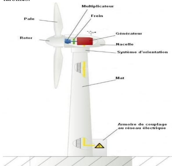
Figure-1: Schematic of a wind turbine
