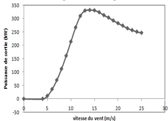
Figure-7: Effect of wind speed on the output power [1]
