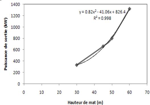
Figure-4: Effect of tower height on the output power [1]
